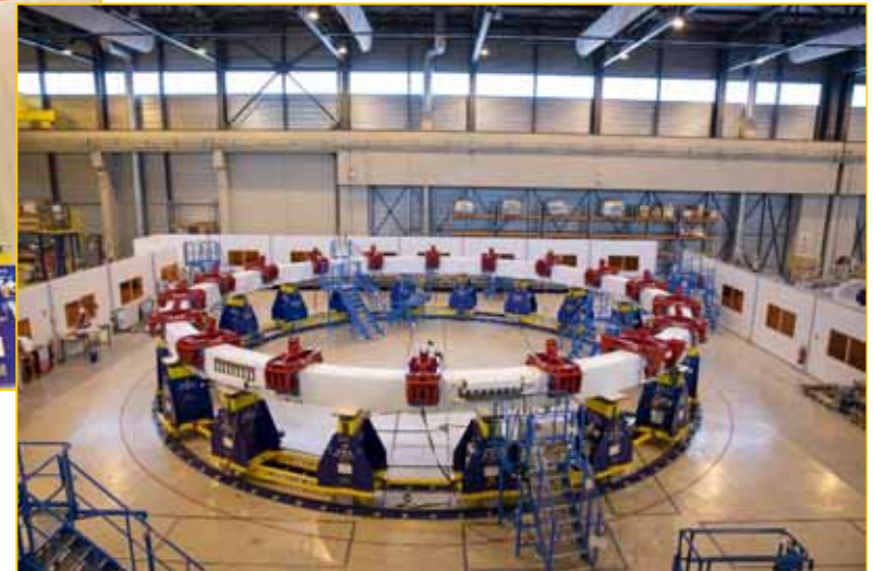
PF Coil #2 ready for resin impregnation, June 2020
